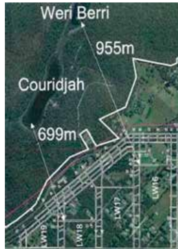
Thirlmere Lakes are not far from Bargo Colliery, close enough for the mine to drain the lakes.
